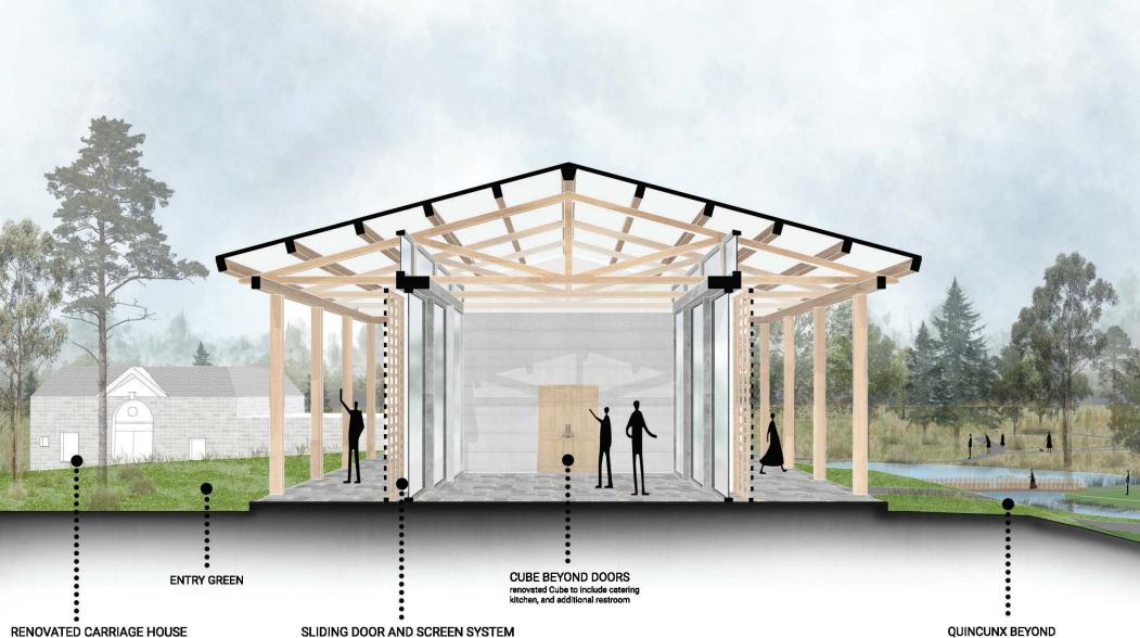
to include display spaces, education wall, and additional storage space SLIDING DOOR AND SCREEN SYSTEM double door system with sliding wood screens on one track and full height glass sliding doors behind
