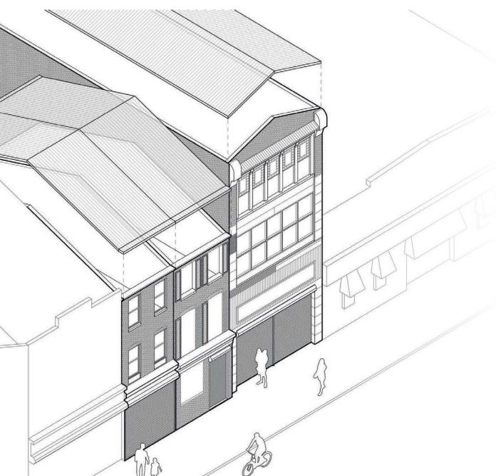
Detailed axonometric of 517, 519 and 521 Old Town Mall; new proposed roofing after renovations.
